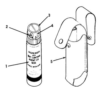
Container (1) contains the CR agent solution, charged to a pressure of 140 psi. The nozzle (2) directs the stream of CR solution. The actuator (3) controls and release of CR agent solution through the nozzle. The actuator has two posi-
