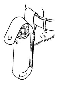
b. Grasp the carrier flap and release the snap button.
