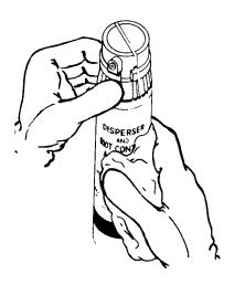
c. Lock actuator and wipe the surface with paper towels or cloth. Throw used paper towels or cloth in drum.
