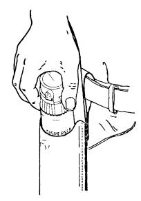
c. Remove the disperser from the carrier.
