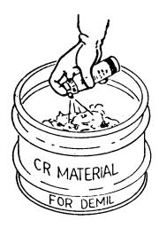
b. To prevent splashing, place towels or cloth in bottom of drum. Unlock actuator, invert the disperser, and discharge the remaining pressure into drum.
