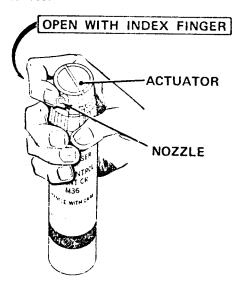
e. Using index finger, rotate the actuator nozzle counterclockwise. This will unlock the actuator.
