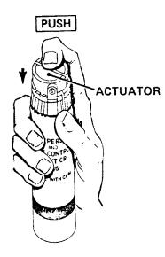
g. Press actuator down with index finger to discharge agent. Use short 1-second bursts or continuous stream as required.
